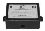
The VZ-ISNSE is a 240V AC power sense module that provides automatic on/off control of a fan or exhaust fan system. The unit detects the current of the circuit to an appliance, ie. clothes dryer, closing and opening the relay when the load sense range parameters are met.
