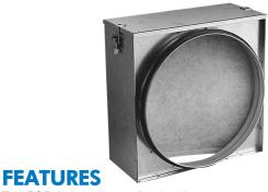
The FGR filter units are fitted with a throw-away panel dust filter. The cassette is made of galvanised steel with rubber-sealed circular connections and the cover has quick-release latches.
