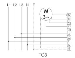
If the motor is protected by thermal overloads and the 2 x TK terminals are not used, they must have a link fitted between them.
