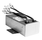
The AVA3.0 controller will vary the speed of 240V AC single phase fan motors in response to DC input signals such as 2 to 20 milliamps or 0 to 10 volts. A potentiometer may be used in lieu of input signals to provide manual control when in 0-10V control. A model that includes an IP55 rated enclosure is available.
