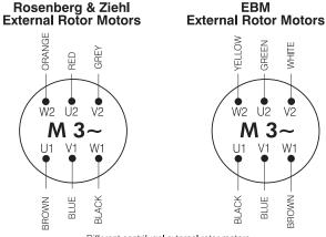
Different centrifugal external rotor motors fans can have different coloured leads as shown
