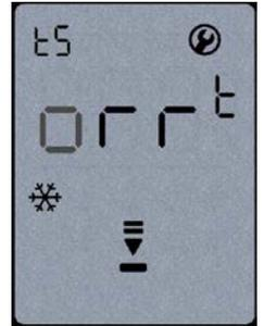
On pressing enter again the three characters will flash until the system has accepted the new setup. Should a capital **E** character be displayed, it indicates an **ERROR** as the setup could not be done on the device being selected. Typically the **o** was chosen for 'on-board' sensing or set point, but an on-board controller is not installed in that control zone. Repeat with the correct selection of parameters. Press the Function button to exit this function.
