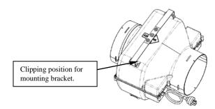
B). Utilise the four holes and four screws provided to fix the fan appropriately.
