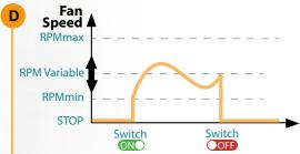
Operating with external on/off switch, the speed can be manually adjusted via an external Potentiometer or 0-10V or 4-20mA signal.
