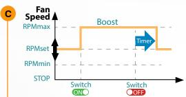
As per B, with an adjustable 1-30min run on time once the external switch has been turned off.
