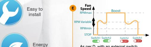
As per D, with an external switch for operation at RPMmax.
