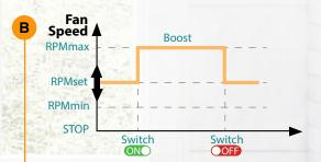
Operating continuously at a predetermined speed between RPMmin & RPMmax, set by internal potentiometer, and going to RPMmax when external switch is turned on.
