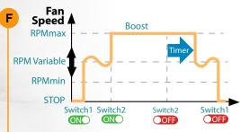
As per E, with an adjustable 1-30min run on time once the external switch has been turned off.
