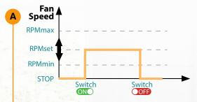
Operating with external on/off switch at a predetermined speed between RPMmin & RPMmax, set by internal potentiometer.
