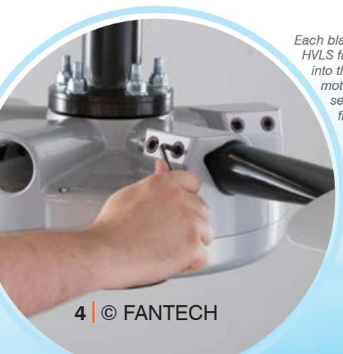
*Each blade on the Titan HVLS fan snap-locks into the direct drive motor hub and is secured via 2 fixing screws*
