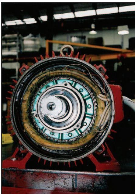
Motor windings being fitted with a set of thermistors.
