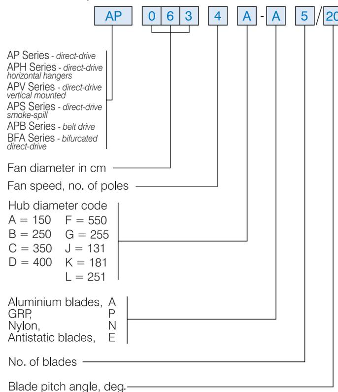
The Fans by Fantech Selection Program is the simplest way to complete a fan selection and generate the product code. It will also providing all options, performance details and dimensional information.
