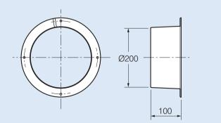
The Inlet Spigot, IS20T, is designed for applications where ducting is required. Care should be taken when installing ductwork as neither the spigot nor the roof unit base is designed for weight-bearing.
