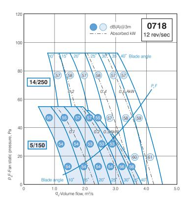
Selecting from these graphs provides a guide only to possible selections. Basic noise level data as well as indicative power absorbed figures are incorporated on the graphs. The Fans by Fantech Product Selection Program will show other possible impeller combinations between the two illustrated here for each fan size/speed. The Selection Program will provide full performance information including air flow, pressure, noise levels, absorbed power as well as complete dimensional information.
