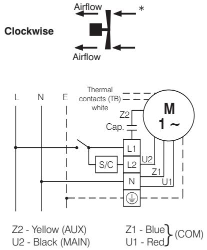
Bridge L1 and L2 if speed controller (S/C) is not required
