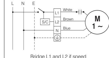
Bridge L1 and L2 if speed controller (S/C) is not required
