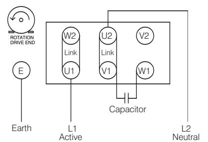
NOTE: W1 and W2 is used for EMT and FASCO motors, replace with Z1 and Z2 for CMG and Tech Top motors.
