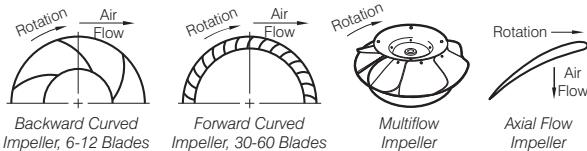
The correct rotation and direction of air flow is shown on each individual fan. If backward-curved centrifugal fans rotate in the wrong direction, the motor may overload and the motor warranty will be void.
