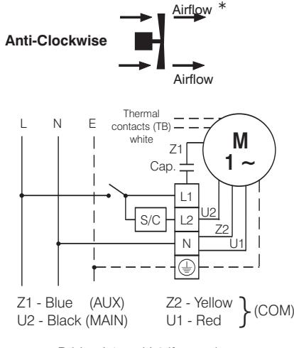
Bridge L1 and L2 if speed controller (S/C) is not required
